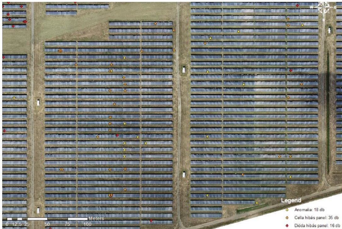
Image 3. Detail of the thermal fault detection results of a solar farm.
